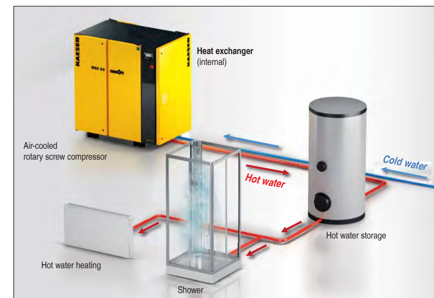
Fig. 3: Heat recovery process
