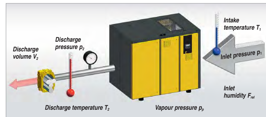
Fig. 1: Free air delivery as per ISO 1217, Appendix C (DIN 1945, Appendix F)
