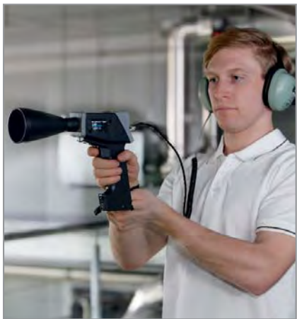
Fig. 4: Leakage location using ultrasound
